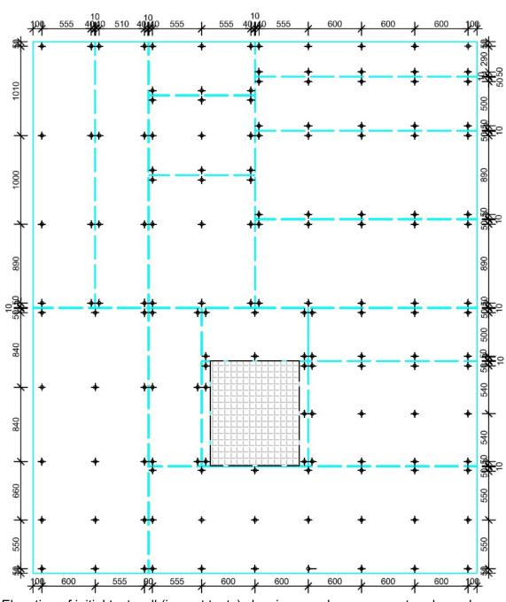
Elevation of initial test wall (impact tests) showing panel arrangement and panel fixing locations
